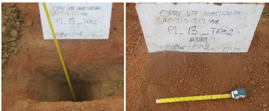
Figure 7-1 Some Test Pit Excavations during Materials Investigation
