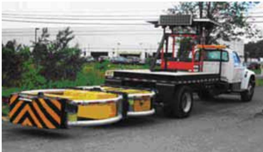
Plate 12.62 TMA with Energy-Absorbing Cartridge
