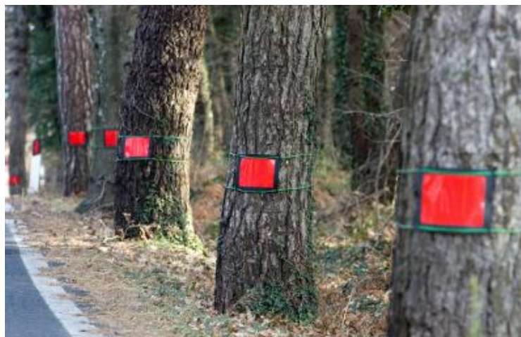
Plate 5.34 Delineation of trees with reflectors
