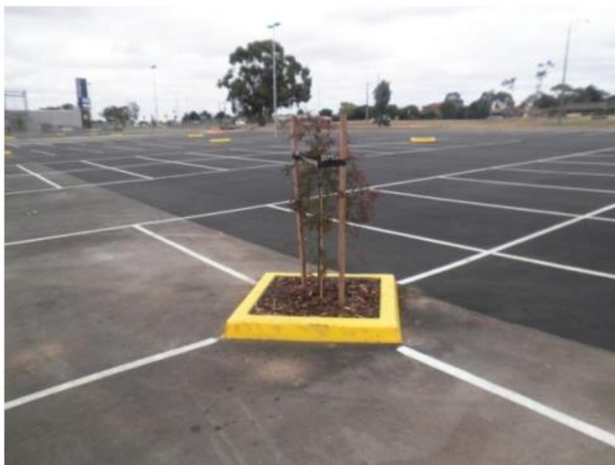
Plate 11.5 Tree planting area too small and inappropriate for traffic safety
