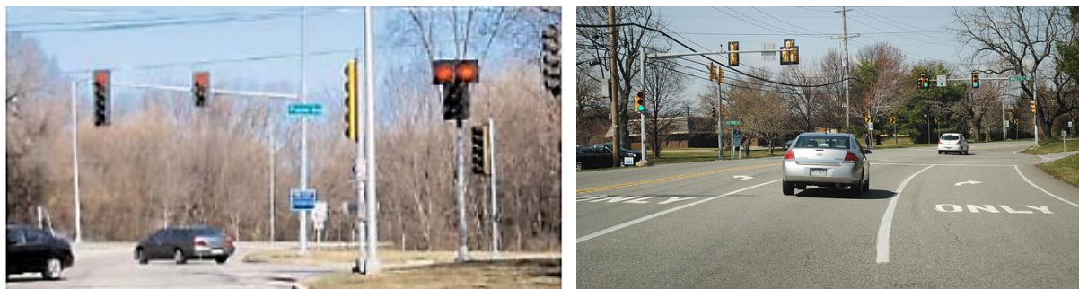
Plate 5.50 Supplemental signal for intersection around a curve
