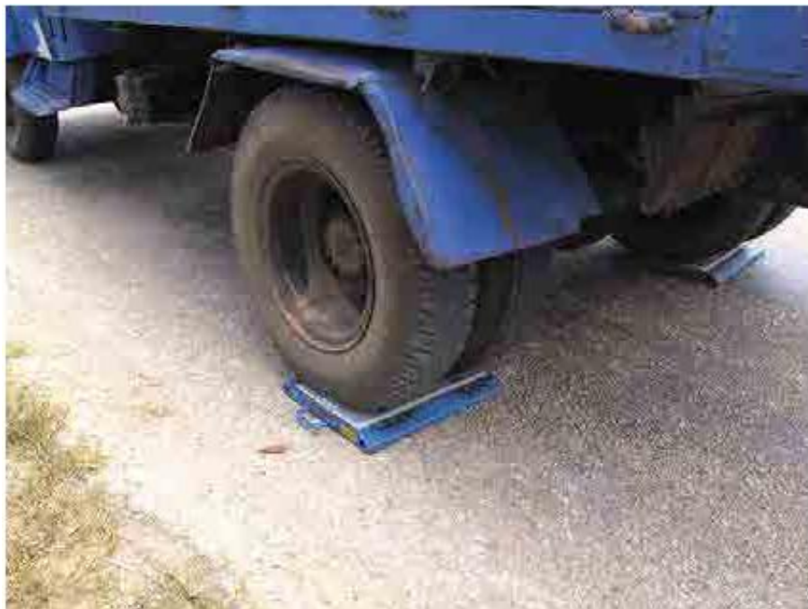
Plate 11.13 Portable Static Weighing Device
