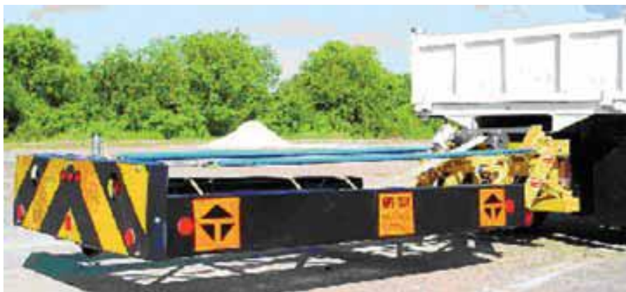
Plate 12.63 TMA with Telescoping Steel Frame and Cutter Assembly
