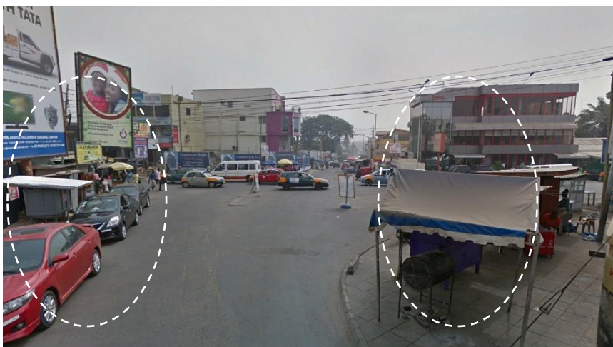
Plate 5.49 Sight triangle obstacle from minor road at cross intersection
