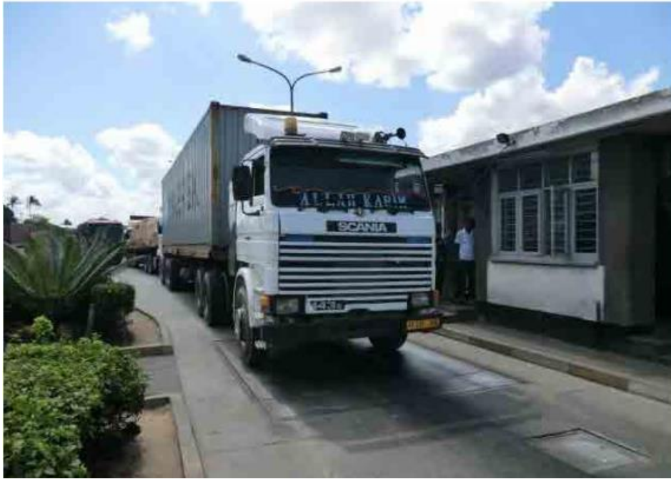
Plate 11.11 Typical 3.2 m × 4 m Axle Unit Scale
