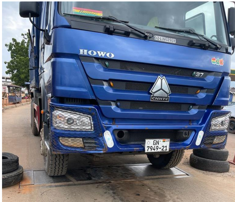
Plate 11.12 3.2 m × 1 m Single Axle Scale
