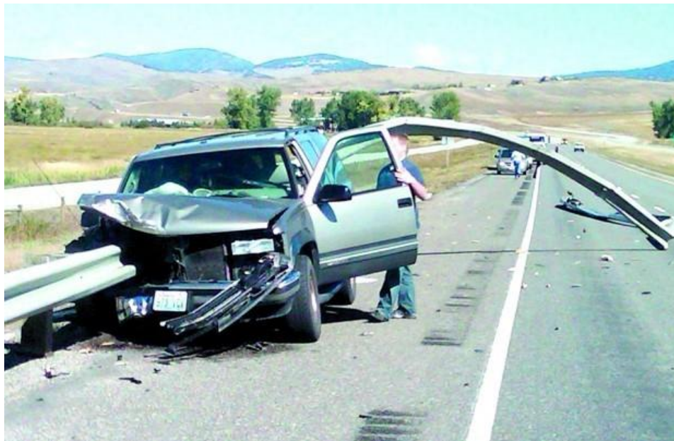
Plate 5.37 Guardrail spearing through an errant vehicle
