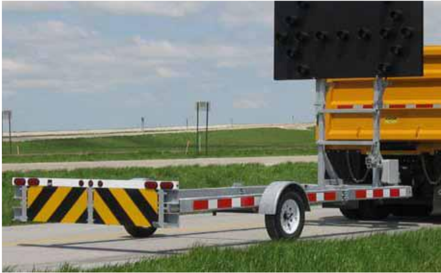
Plate 12.64 TMA with Steel Frame and Burster or Kinker Assembly
