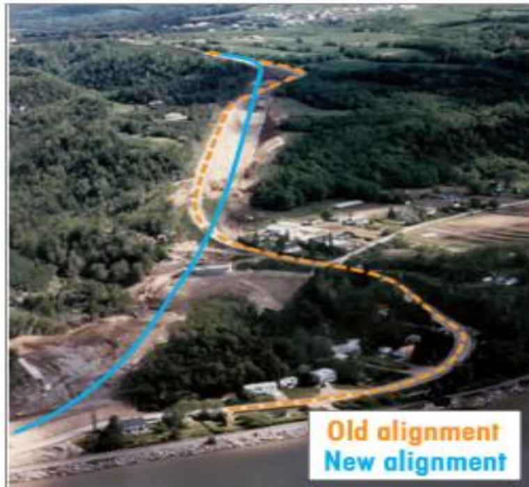
Plate 5.31 Alignment modification to eliminate a sharp curve at the bottom of a steep grade.
