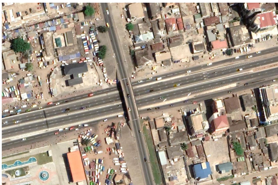
Plate 5.56 A sample overpass with no connection between two routes
